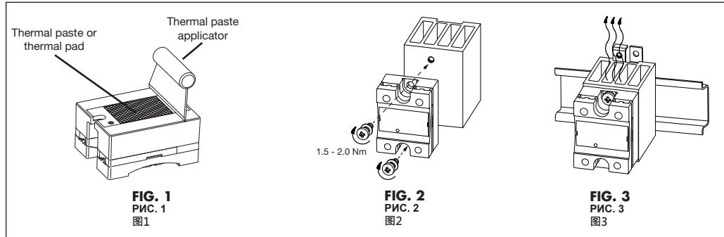
**FIG. 1:** A thermal interface is required between SSR and mounting surface. Thermally conductive silicone paste shall be applied and spread throughout the base of the SSR. Alternatively, a thermal pad shall be affixed to the baseplate of the SSR before mounting the SSR on the heatsink.
