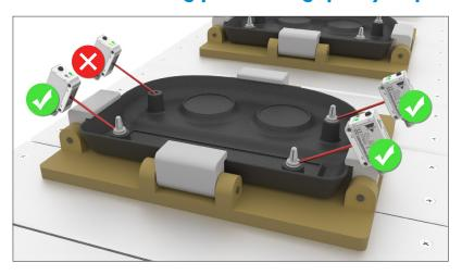
The small 1 mm visible round red laser spots are aligned on the background surface with the clips missing and taught in foreground suppression mode to recognize the background itself. If the clips are correctly mounted, they will prevent the sensor from seeing the background and thus the clips are detected.
