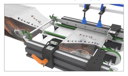
The small 1 mm round laser spots are easy to align so the setting of the guides can be adjusted correctly. The sensors have been taught in foreground suppression mode to detect a background below the conveyor, allowing reliable detection of pouches, regardless of whether all laser light is reflected away from the sensor or absorbed by a dead black pouch.
