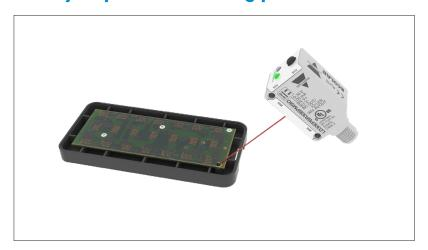
The 1 mm, visible, round, red laser spot is aimed at the background surface with the small screw missing, and the sensor taught in Dual Detection mode to recognize the background. If the screw has been correctly mounted, it will block the sensor from seeing the background, and the small screw will be detected.
