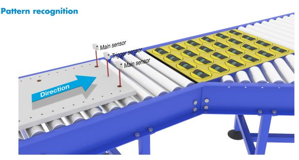
The pattern recognition function is used to verify if a manufactured part has all the e.g. holes or taps as expected and that the parts are made according to the specification.
