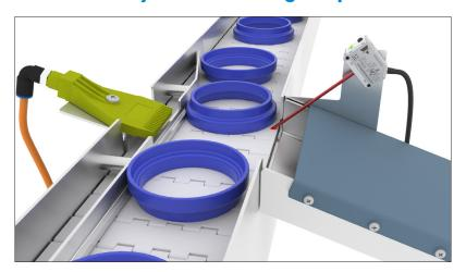
The small 1 mm visible round red laser spot is aligned on the white conveying belt and taught in foreground suppression mode to recognize the belt. If a part is turned upside down and hence its larger diameter lying directly on the belt is blocking the sensor from seeing the belt, the blow nozzle is triggered and sends the part back into the vibratory bowl.
